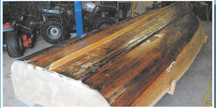
Seal coat and prep for finish
