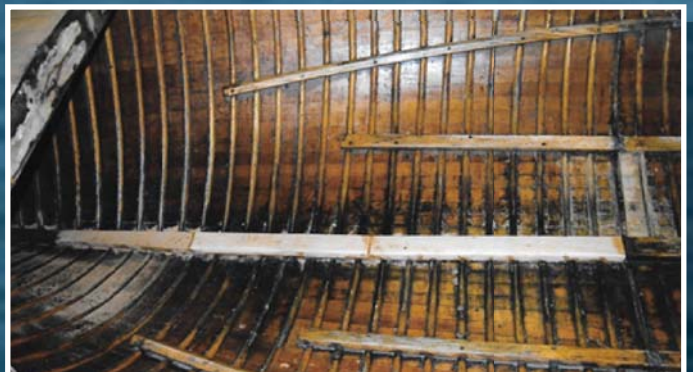
Replacing parts of keelson with white oak
