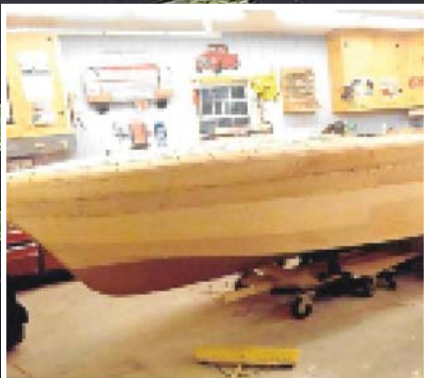
New planks installed and sanded for varnish.
