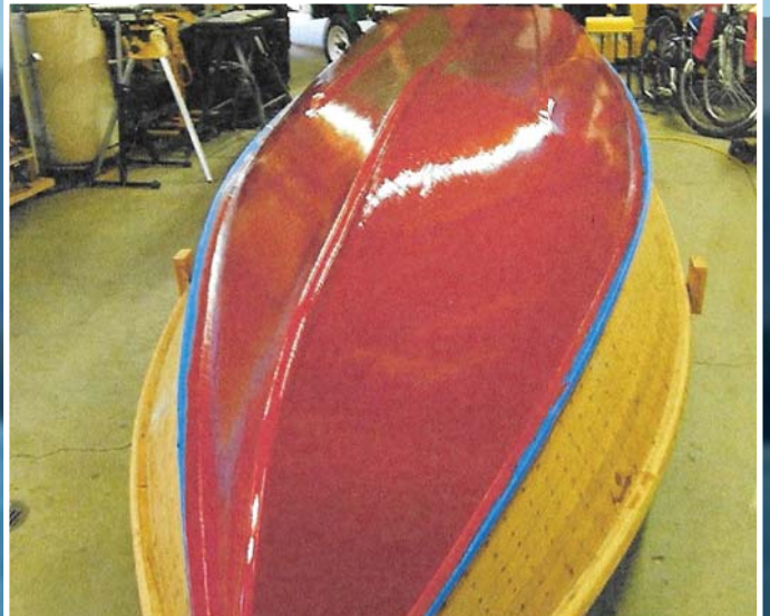
Two coats of red epoxy paint
