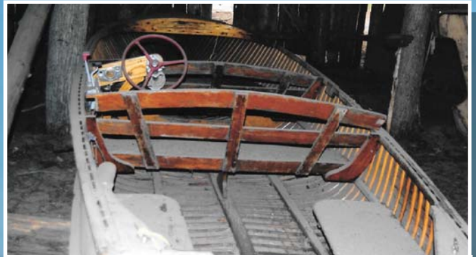
Interior deterioration after many years storage
