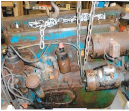
Engine being removed for rebuilding.
