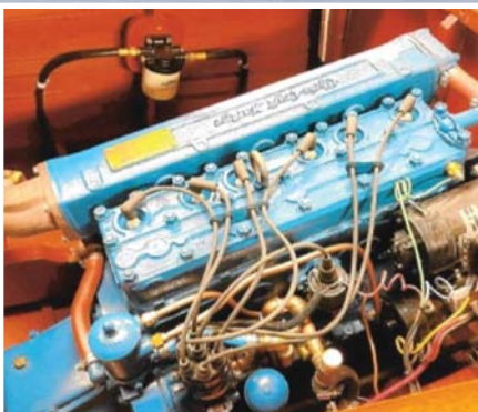
Engine after rebuilding and installation.
